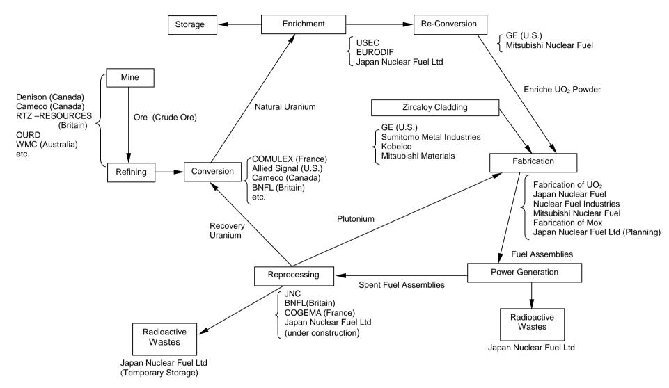
FIG. 6. Nuclear Fuel Cycle Diagram
